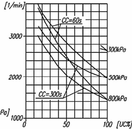
**NOTE!** The above characteristics are for open-inlet-valve control system at minimum cooling requirements and at ambient temperature +20°C
